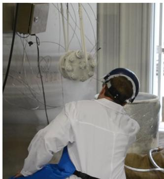
Earlier this quarter, Hy-Grade Valve took delivery of our recently purchased Cryogenic Testing Unit produced by Ventil. The unit uses liquid nitrogen to cool valves to temperatures as low as -196 degrees Celcius Then, gaseous helium is pumped through the valves and a specialized “sniffer” is used to test for leakage in parts per million (PPM). The machine sits alongside our standard hydrostatic
